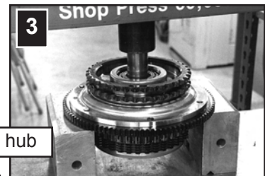
Press until the hub bottoms.
