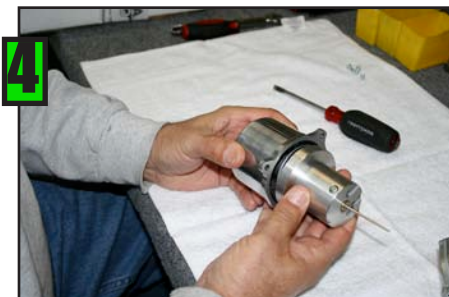
4 Remove Piston from Dome.
