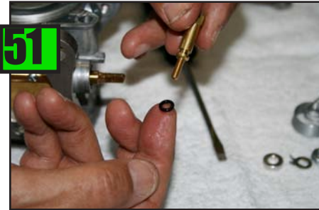
Remove Idle Speed Screw oring.
