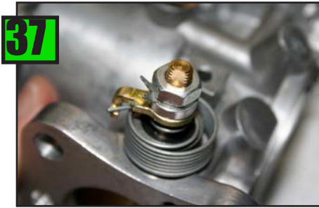
With tabs bent back prepare to remove nut.
