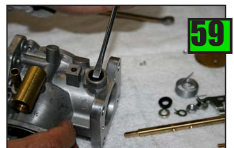
Both Throttle Spindle Shaft seals should be removed.
