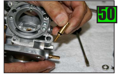
Idle Speed screw removed.
