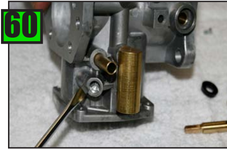
Remove Main Jet Adjusting Screw.
