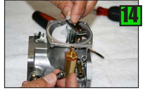
Remove screw from Bi-Metallic Lever & lift straight up.
