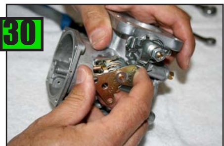
Lift up and remove Choke Cam Lever.
