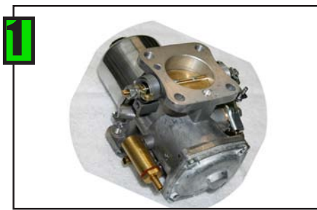
1 SU Eliminator II Carb ready for disassembly.
