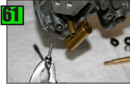
Main Jet Adjusting Screw removed.
