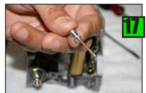
Float Spindle Screw removed.
