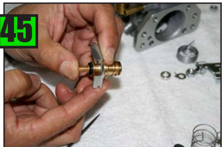
Push the threaded end of Chody Body Spindle outward.
