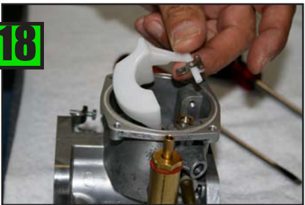
Lift up and remove Float.
