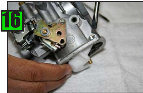
Remove Float Spindle Screw.
