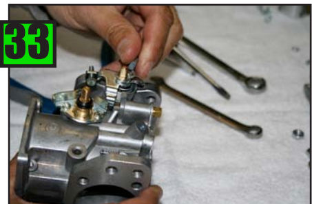
Bend lock tabs back and remove nut from Idle Stop Lever.
