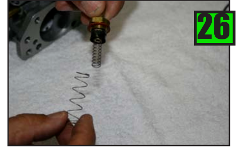
Remove large Tickler Spring from Tickler Pump Assy..
