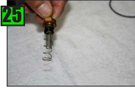
Tickler Pump Assy. removed from Ticker Body.
