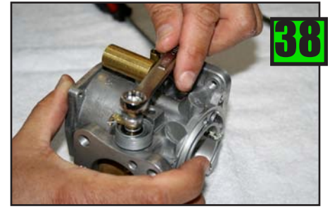
Remove nut from Spring Retainer with 7/16" wrench.
