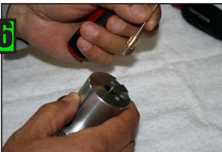
6 Remove Needle from Piston.
