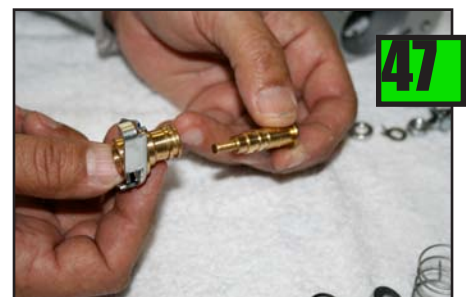
Remove spindle from Choke Body..
