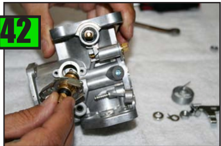
Lift up and remove Choke Body.
