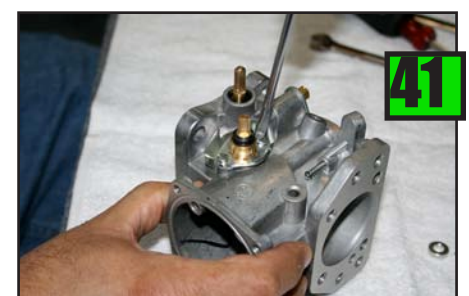
Next remove the (2) Choke Body Screws.
