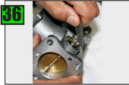
Bend lock tabs back on Throttle Spring Retainer.
