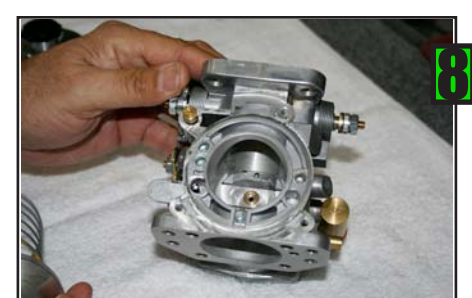
8 Body with Piston removed.
