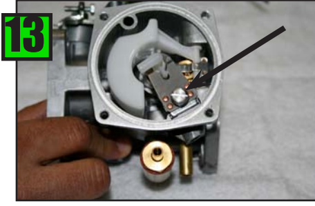
Remove Bi-Metallic Lever & Main Jet.
