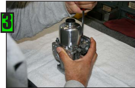
3 Remove (3) Dome screws.
