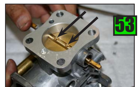
Next remove the (2) Throttle Blade Screws.
