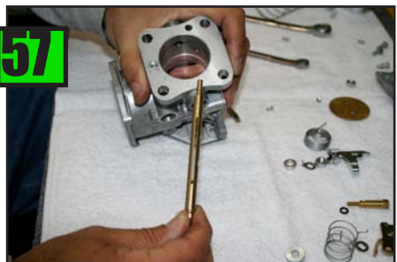
Throttle Shaft removed.
