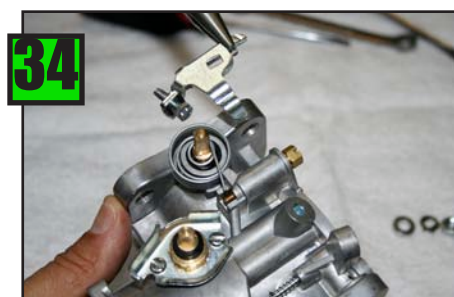
Remove Idle Stop Lever and Throttle Return Spring.
