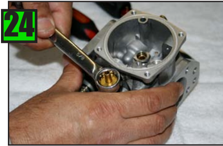
Disassemble Ticker Pump Body.
