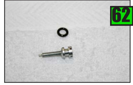
Main Jet Adjusting Screw & oring.
