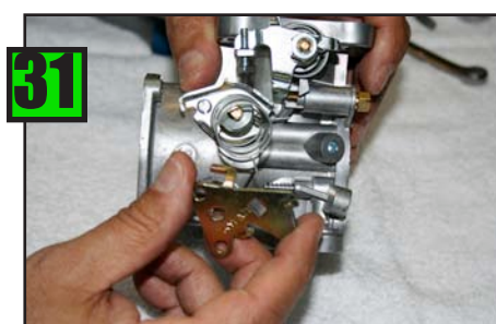
Remove Choke Spring.
