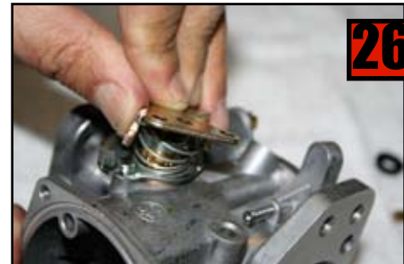
Install Choke Cam Lever.
