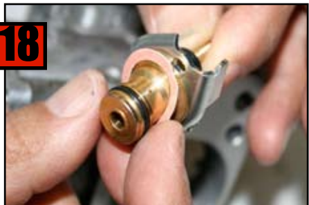
18 Match slot in gasket to locating hole in Choke Body.
