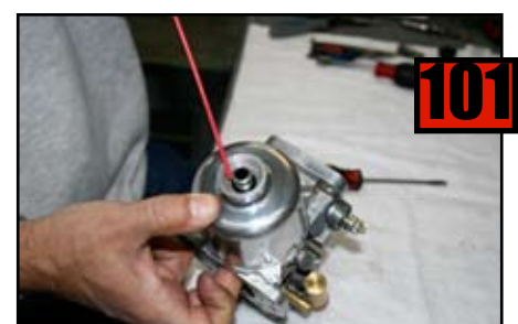
Spray a small amount of WD in top of Dome onto the piston.
