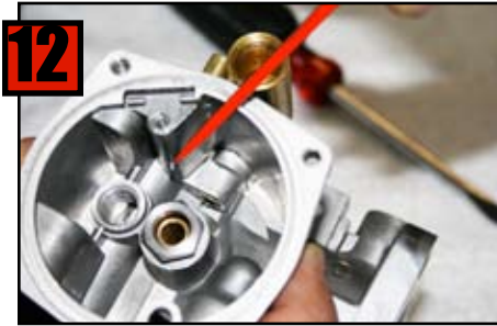
12 Thread Main Jet Adjusting Screw in til you see the end.
