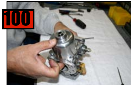
After securing the Dome, insure that Piston moves freely.
