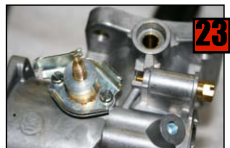
23 Place dust cap on installed Choke Body.
