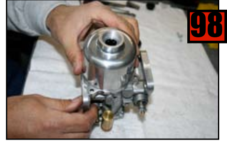
The Dome can only be put on one way for all 3 holes to align.
