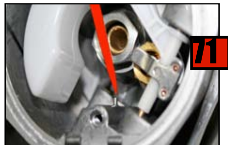
End of Main Jet Adj. Screw lines up with Bi-metallic Lever.
