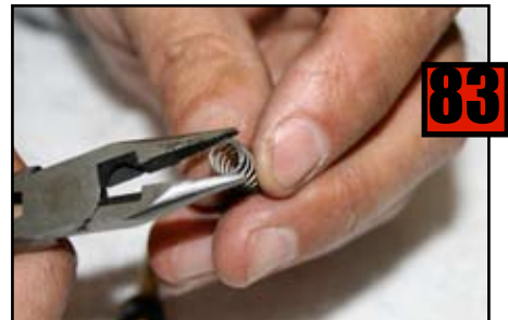
Squeeze end of small Tickler Spring so it will stay on Stem.
