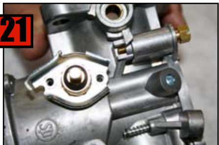
21 Choke Body lined up with screw holes.
