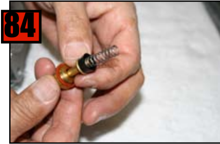
Slide the Tickler Stem with Viton Cup & Spring into Nut.
