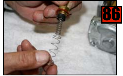
Install Large Spring over Small Spring.
