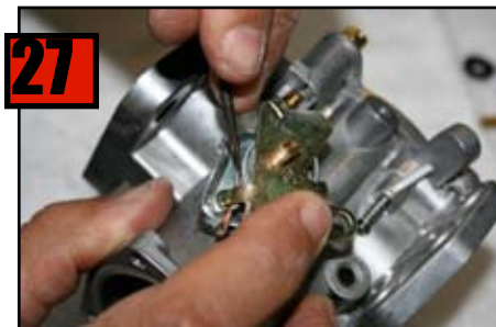
Line up spring coils close to Choke Body.
