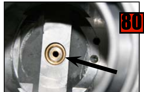
Set the Main Jet so that it is flush with the seat bevel.
