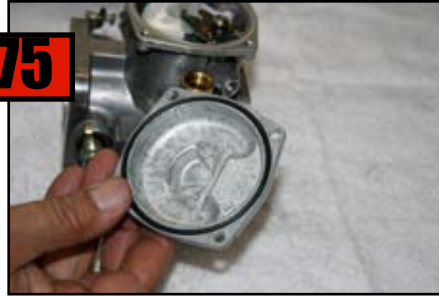
Place oring into Float Bowl Cover.
