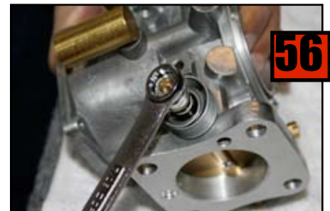
Tighten nut onto Throttle Return Spring Retainer.
