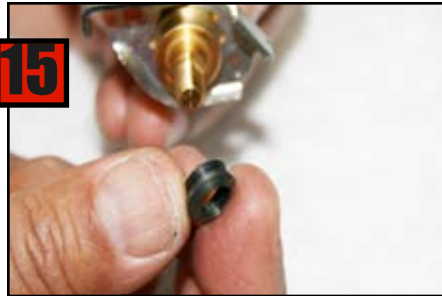
15 Place open end of seal on spindle first.
