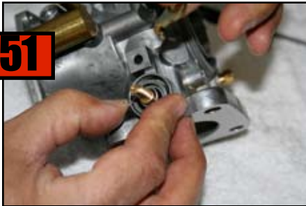
Tension Throttle Return Spring.
