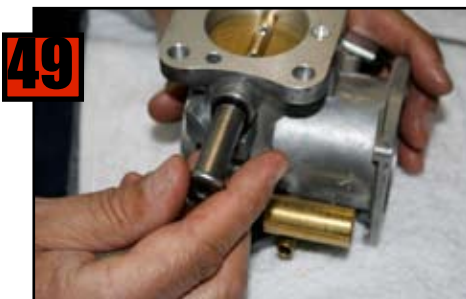
Push the seal in with your homemade tool.
