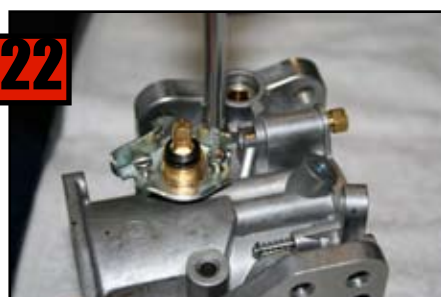
22 Install (2) screws to secure Choke Body.
