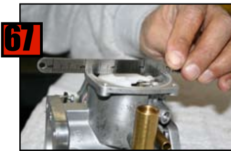
Check Float level and adjust as necessary. See #68.
