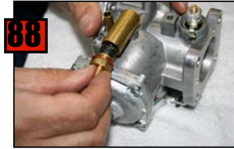
Now insert the Tickler Pump Assy into Tickler Pump Body.
