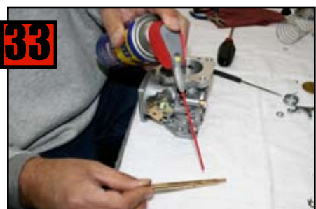
Spray a little WD on Throttle Shaft prior to installing.
