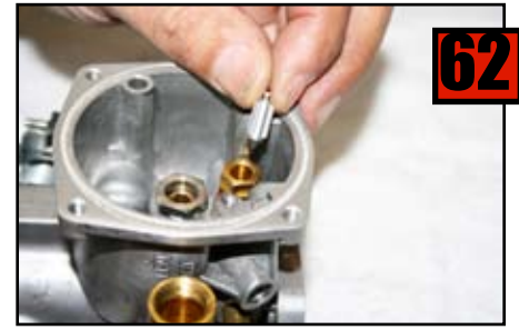
Drop needle into the seat with the rubber tip first in.
