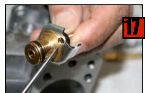
17 Note offset hole in Choke Body where the gasket locates.
