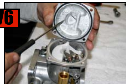
Note the relief for the top of the Main Jet.
