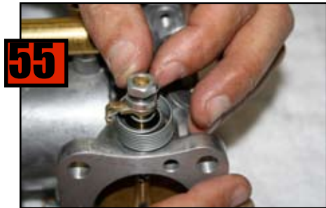
Install nut onto Throttle Return Spring Retainer.
