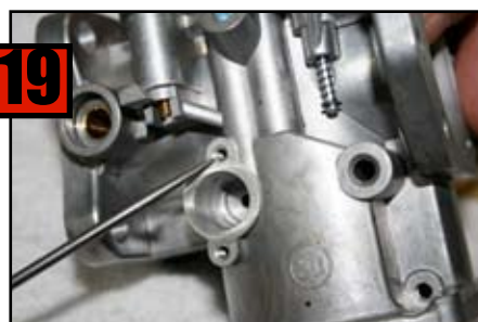
19 Note offset hole in body lines up with hole in Choke Body.
