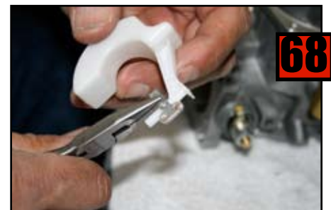
Bend Float tab to adjust Float level as needed.
