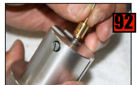
Install Jet Needle Ay. with Guide slot facing Screw.
