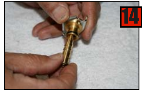
14 Install spindle into Choke Body threads first.
