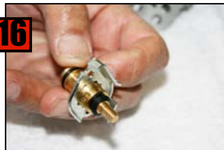
16 Choke Body ready for installation.
