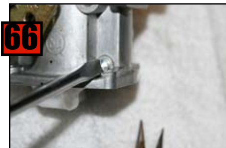
Tighten Float Spindle Screw with blade type screwdriver.
