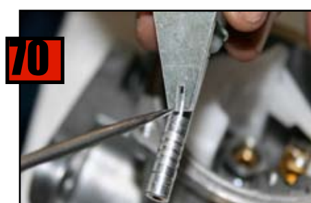
Note slot at bottom of Bi-metallic Lever for main jet adj. screw
