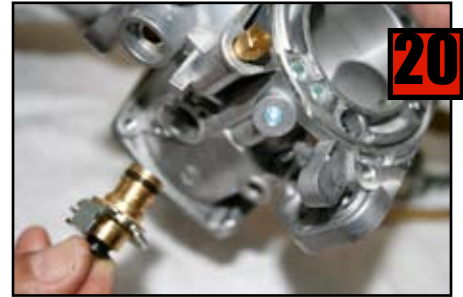
20 Now place Choke Body in carb body.
