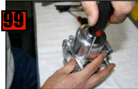
Align all 3 holes, then fasten Dome to body with 3 screws.
