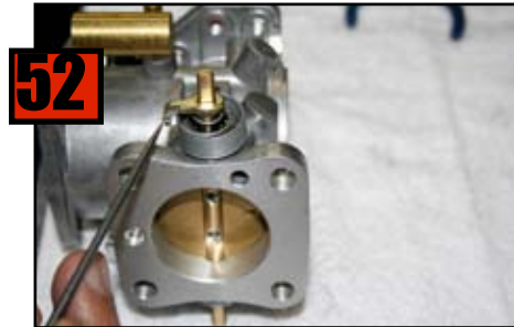
Engage Throttle Return Spring onto Spring Retainer.
