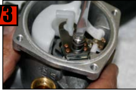
Use the Screw & Spring to hold down Bi-metallic Lever.
