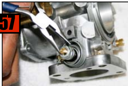
Bend locktabs to secure nut.
