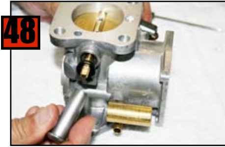
Now install LS Throttle Shaft seal.
