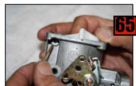
Position Float Spindle Screw for installation.
