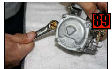
Hand tighten, then tighten with a 5/8" wrench.
