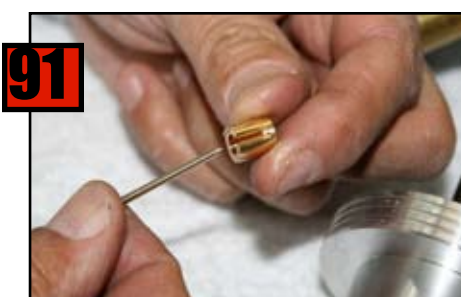
Install Jet Needle Guide on Jet Needle as shown.
