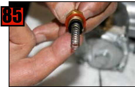
Put small amount of lube on Viton Cup to ease installation.
