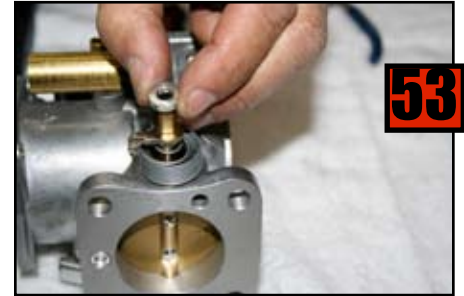
Install spacer onto Throttle Return Spring Retainer.
