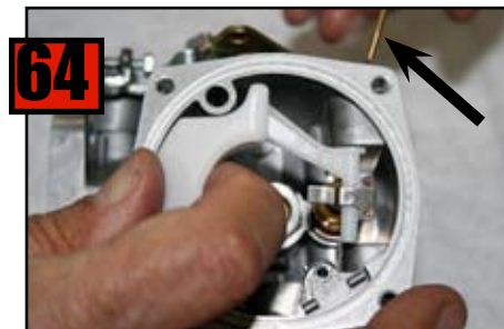
Now position float for installation of Float Spindle Screw.
