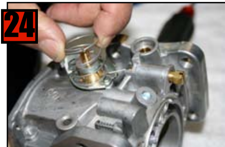
Install spring on Choke Body.
