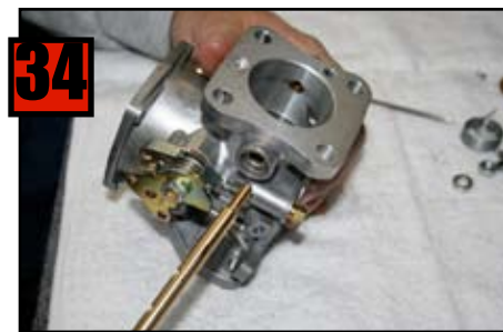
Align Throttle Shaft with Shaft hole in body.
