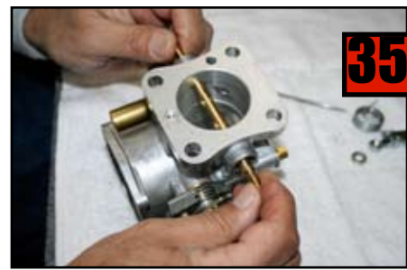
Slide Throttle Shaft through both shaft holes in body.
