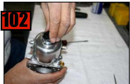
Install Dome cap snuging it up by hand only!
