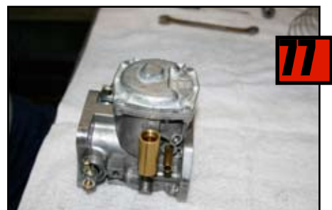
Float Bowl Cover in place for installation.
