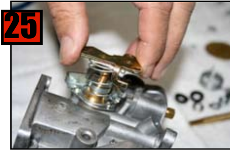
Locate spring on Choke Cam Lever.
