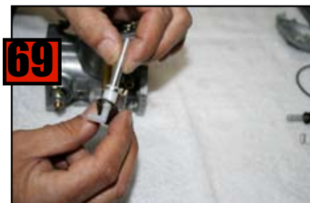
Install Bi-Metallic Lever onto Main Jet as shown.
