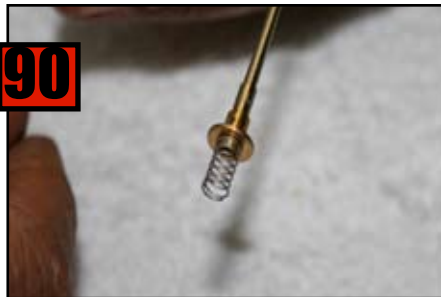
Install Jet Needle Spring on blunt end of Jet Needle.
