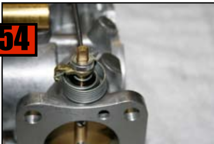
Install locktab onto Throttle Return Spring Retainer.
