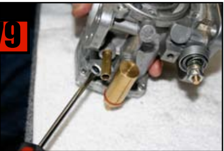
Adjust the Main Jet Adjusting Screw to set the Main Jet.
