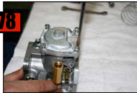
Install Float Bowl Cover with (4) screws & lock washers.
