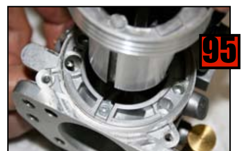
Now install the Piston with slot facing the Piston Guide.
