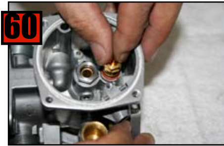
Thread the Seat in by hand.
