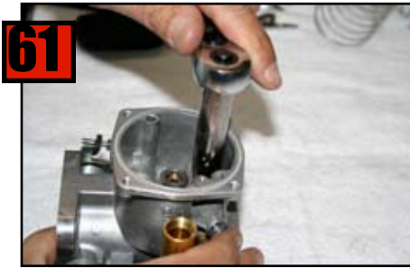
Use 7/16" deep socket to tighten Seat in place.
