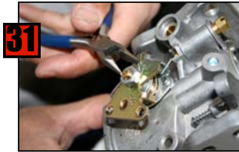
Bend lock tabs to secure nut.
