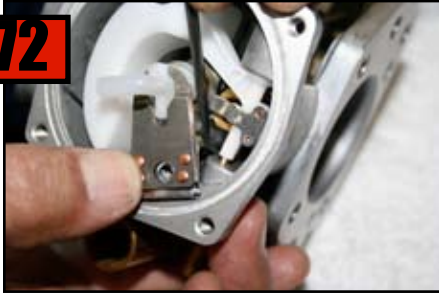
Note that slot in Lever and end of Adjusting screw are aligned.
