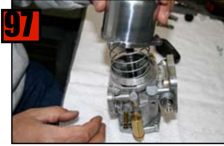
Position the Dome over the spring & slide it down.
